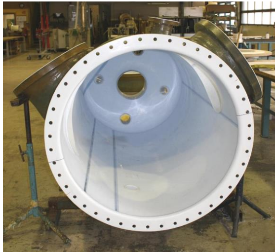
Fluoropolymer linings of FRP systems to ensure ultra-high-purity of chemicals used for chip manufacturing through production, storage, transportation and usage.
