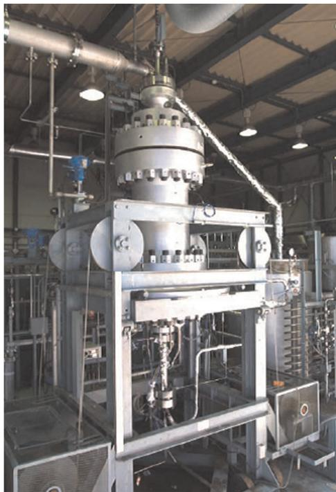
Fig. 20 Industrial supercritical water reactor for organic solvent treatment. This flow reactor can treat 1 metric tonnes waste per day. (This photograph was kindly provided by Organo Corporation (Tokyo). Permission for use was obtained from the company.)
