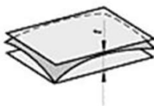
Figure 1 Edge waviness (from DIN ISO 1101 (University Essen / Duisburg, ipe))
