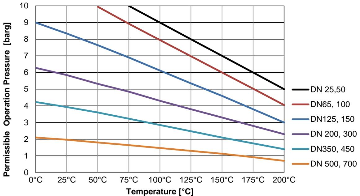
Fig. 8: Minimum pressure resistance of two- and three-convolution PTFE-expansion joints, including safety factor 2
