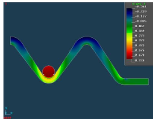
Fig. 4b: FEM Calculation of tangential stress
