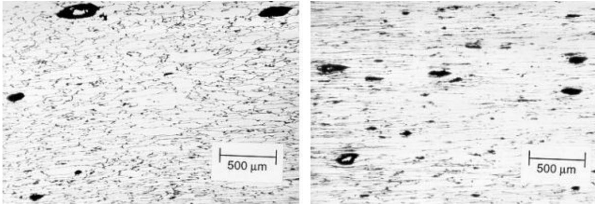
Fig. 7a and 7b: Inhomogeneous distribution, does not comply with the requirements
