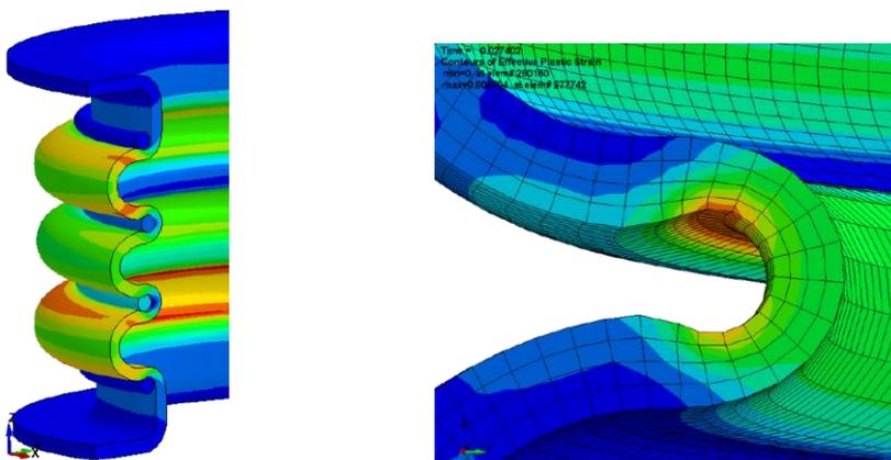
Fig. 9a and b: Simulation of the maximal operation pressure before plastic deformation; Source SGL / Dr. Schnabel GmbH
