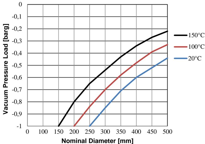
Fig. 10: Vacuum resistance of two- and three-convolution PTFE-expansion joints
