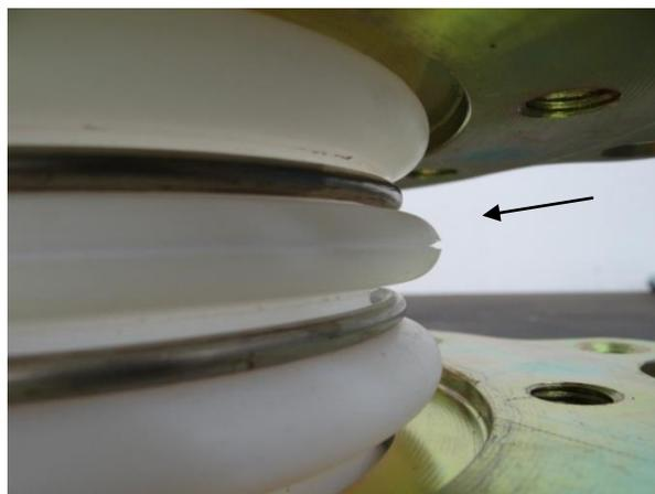
Fig. 5: Crack initiation after <5000 axial movement cycles due to an inhomogeneous distribution of the wall thickness
