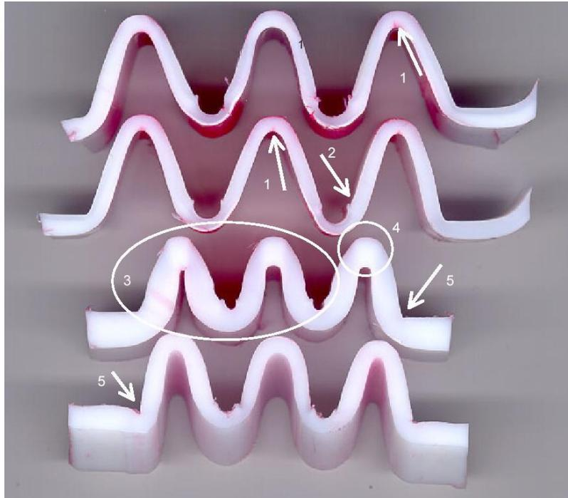
**Fig. 2: Unacceptable defects that reduce the performance of the PTFE bellow**
