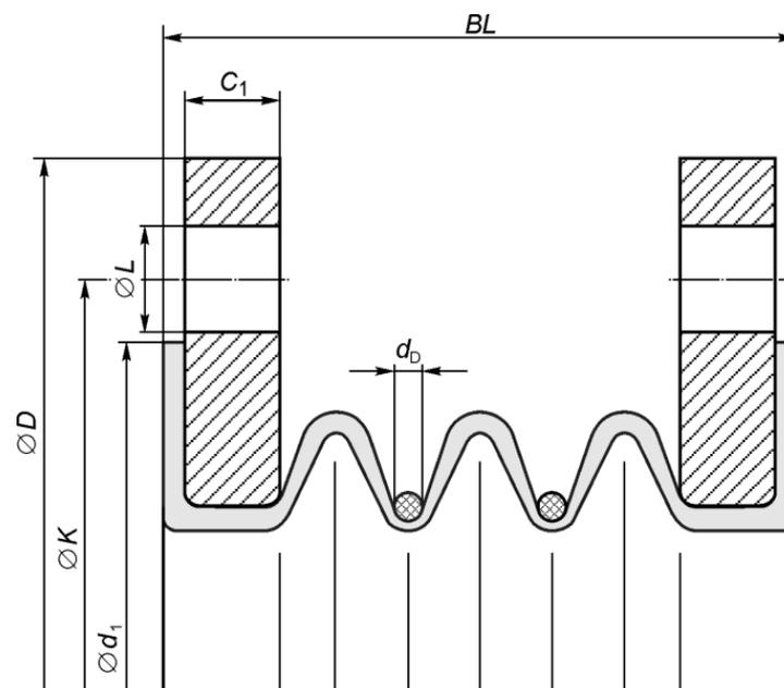
Fig. 11: Design of a PTFE-axial expansion joint; example for a three convolution layout
