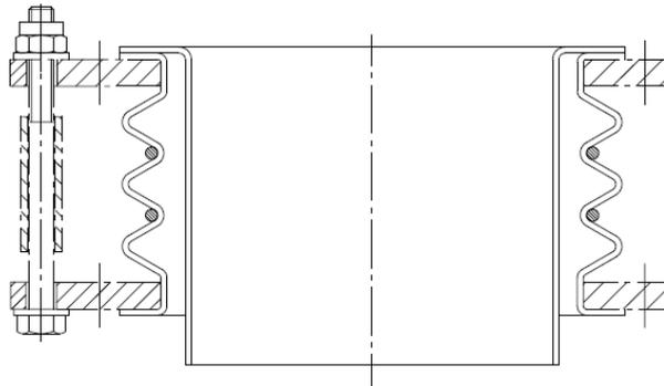
Fig 15: Expansion joint with smoothbore protection sleeve
