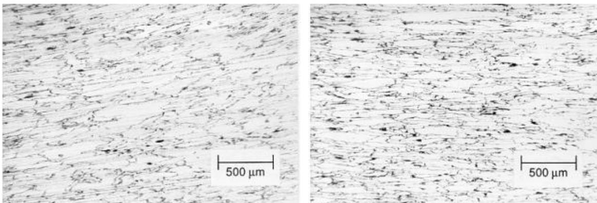
Fig. 6a and 6b: Homogeneous distribution of antistatic modifier
